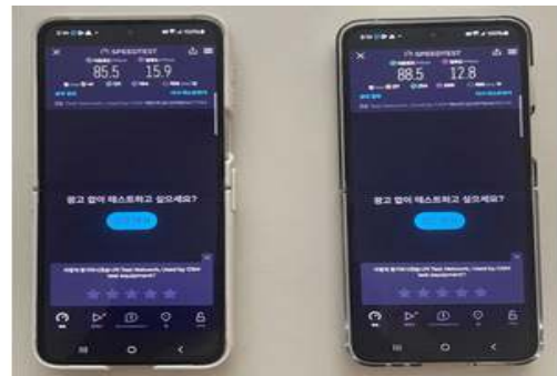
Speedtest 측정 결과(동시): Download/Upload=85.5/15.9Mbps
